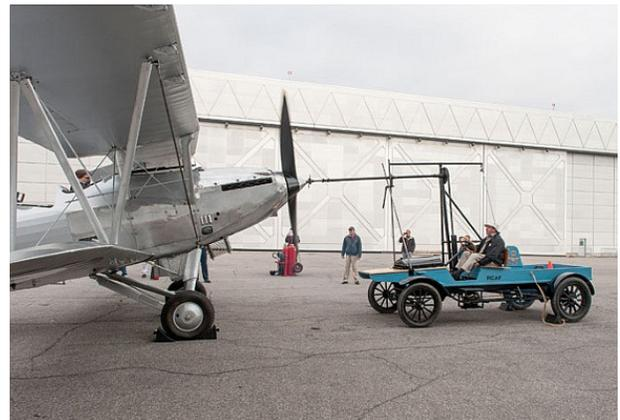
A man in a flight suit stands by the Hind's wingtip, where driver and pilot can both see him. He calls to the pilot, not shouting, but projecting very clearly, “Fuel on? Mixture rich? Throttle set? Mags on? Contact?” and hears the pilot's reply: “Contact!” The flight-suited arm is raised, thumb-up, and then whirled in a circular motion. This is the moment of truth. It happens now.
